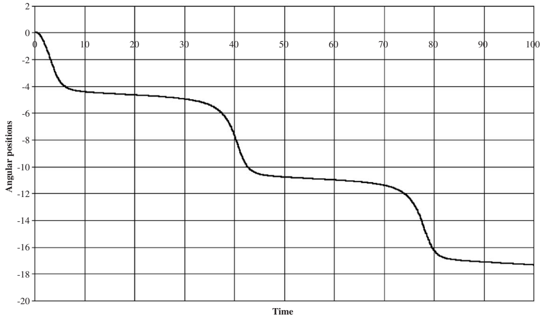
Fig. 12. Variation of angular positions of balls with time, \bar{I} = 0.25 , \nu = 0.05 , A = 0.05 , \Omega = 3.5 (modified initial conditions): —, \psi_1 ; - - - - - , \psi_2 .
